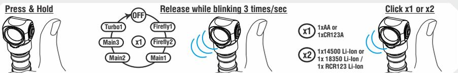
To access the Menu press and hold the switch button (when the flashlight is switched off). It will switch on, go through 6 modes, then after 2sec in Turbo1 mode – enter to Menu and flash about 3 times a second.
