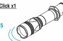
**Momentary on** – any mode switched on by half-pressing of the button (no click!) and active till the button is released. It is suitable for giving signals by short button pressings. Click the button to switch the light on permanently.
